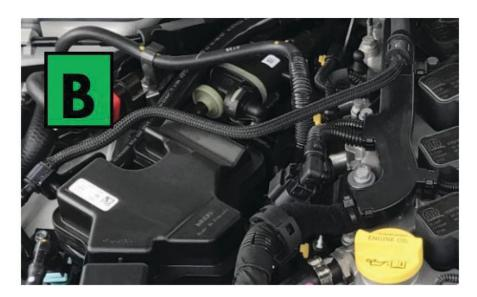
Disconnect the factory Manifold Pressure Sensor from the factory harness.
