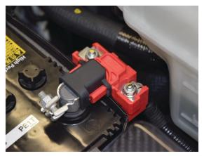
2. Unbolt the 10mm nut and place the positive (red) harness lead to the battery.
